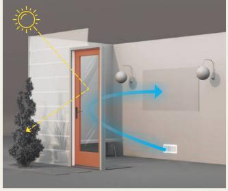
In warm weather, Low-E glass reflects the sun's rays off the glass and a home's air conditioning back inside to help keep the home cool.
